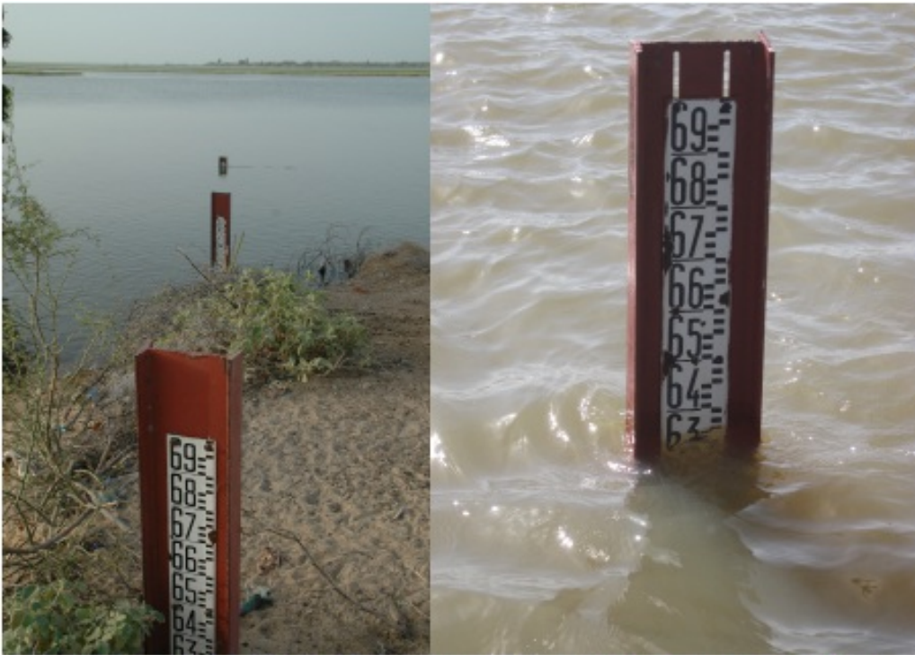
DNH uses sturdy gauges for their daily measurements of the water level in Douna (left) and Sofara (right) and in many other places.
